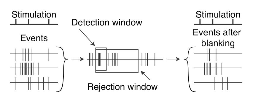
If more than 60% of the channels had spikes within a 400 µs detection window, then all spikes inside the 2 ms rejection window were ignored
