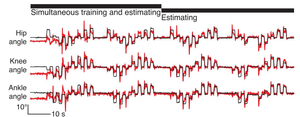
Example of real-time estimation of joint angles during passive movement. During the training phase, the actual joint angles and the neural firing rates were used to continuously update the model. Simultaneously, the decoder used the most recent model to estimate the joint position (red). After the training phase, the final model was used to estimate the kinematics.
