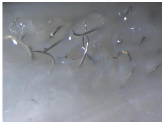
**Figure 8.** Dissection photograph of a poorly placed array. The electrodes tips were driven completely through the root and presumably contacted against the wall of the spinal column during insertion, causing them to bend and break.
