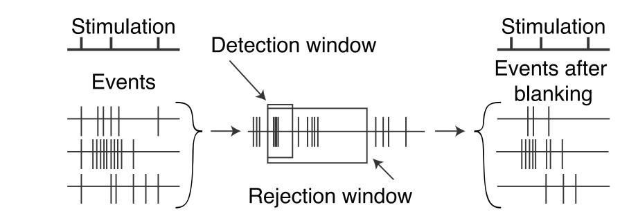
If more than 60% of the channels had spikes within a 400 µs detection window, then all spikes inside the 2 ms rejection window were ignored
