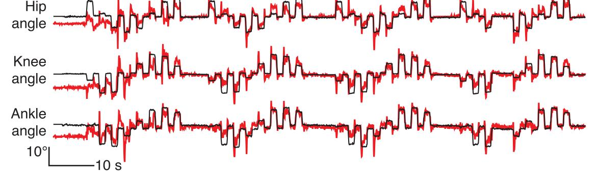
Example of real-time estimation of joint angles during passive movement. During the training phase, the actual joint angles and the neural firing rates were used to continuously update the model. Simultaneously, the decoder used the most recent model to estimate the joint position (red). After the training phase, the final model was used to estimate the kinematics.
